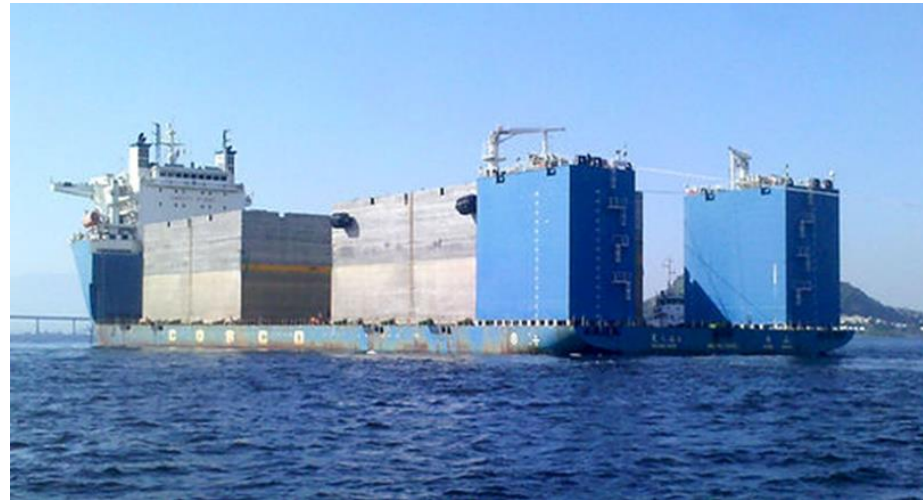
Caisson transportation using semi-submersible vessel
